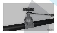
After installation, it is good practice to record the tightening of the bonnet and gland nut. In case of leakage from the stem, simply tighten the gland nut with a spanner. If the leakage continues, the gland nut packing must be replaced.
