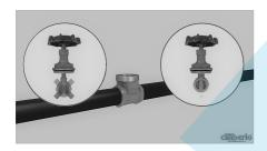
To assemble the bonnet on the gate valve body it is advisable to tighten it gradually to prevent the seal between the two parts from being subjected to excessive stress.
