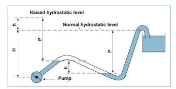
In the same way as in a gravity main, the presence of air pockets is detrimental to the effective performance of a pumping main. In this case, there is a pressure increase h (height h of the additional head to be lifted), which the pump must supply in addition to pressure H in order to compensate for the increased head due to the air pocket, with the hydrostatic level being raised by this value. For the same flow rate, the energy consumption is increased proportionally.
