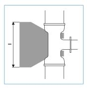
1/16 bend, DN 250 Test pressure: 10 bar Height of cover: 1.2 m
