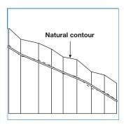
A pipeline layout must be designed to facilitate air accumulation at clearly defined high spots, where purging equipment must be installed.
