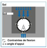
$\begin{aligned} & \text{Bending stresses} \\ & \alpha = \text{bedding angle} \end{aligned}$
