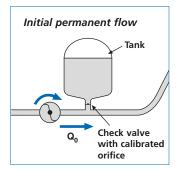
The protective systems that can be installed to limit water hammers to an acceptable level are varied and must be adapted to suit each situation.
