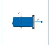
**Hydraulic thrust:** the table below gives the thrust forces at a pressure of 1 bar. (For other pressures, multiply by the site test pressure in bar).
