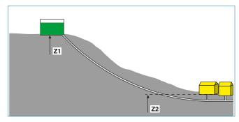
A gravity supply system is the mode of supply which allows water to be driven through a pressure main from a natural or artificial storage area at elevation Z1, to all points of supply located at elevations Z2 < Z1, without any energy input.
