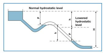
The air pocket transmits static pressure P from its upstream face to the downstream face and the hydrostatic level drops. Operating pressure H is reduced by quantity h, corresponding to the difference in level between the ends of the air pocket and the missing head height.
