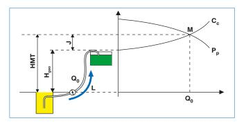
C<sub>c</sub> : pipeline characteristic H : H<sub>geo</sub> + J J = f (Q<sup>2</sup>) P<sub>p</sub> : pump characteristic
